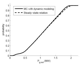
Figure 9: Cumulative distribution function of a 5 turbine wind farm generation obtained with dynamic modeling and steady-state power curve with an annual mean wind speed of 10 m/s.
