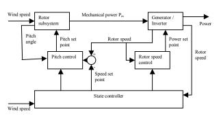
Figure 2: interactions between wind turbine's elements.
