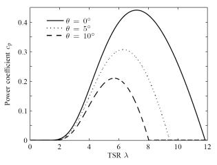
Figure 3: Power coefficient as a function of the tip speed ratio for different pitch angle.
