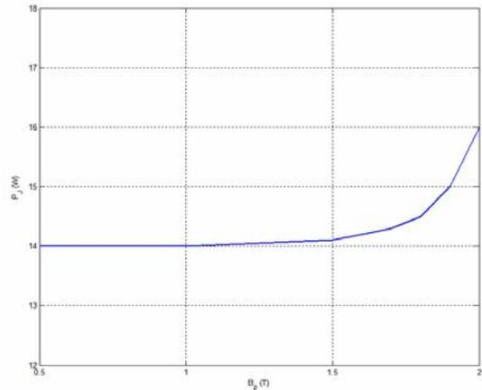
Figure 6 : Copper losses in function of  $B_p$ .
