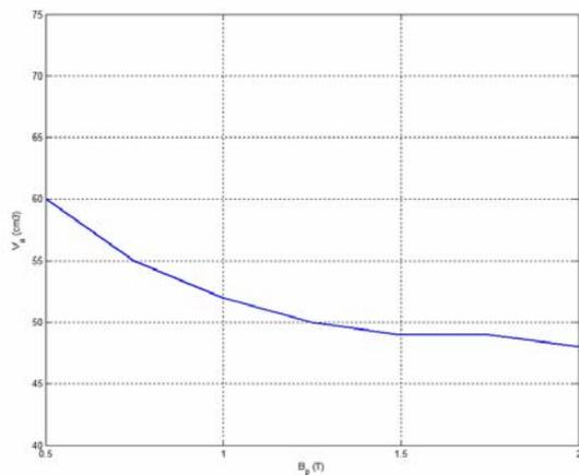
Figure 7 : Actuator volume in function of  $B_p$ .
