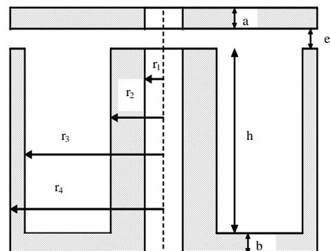
Figure 1 : Cross section of the actuator.
