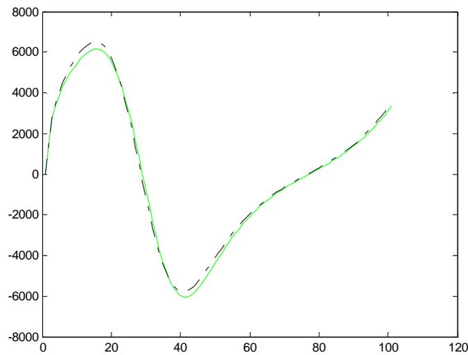
Fig. 2 - Pressure variation at the midpoint of a beam, as it is excited with a periodic force. The maximum amplitude of the displacements of the beam is equal to half the thickness of the fluid film. The dashed line corresponds to the results obtained with a finite difference model ( $55 \times 25$  nodes), whereas the continuous line corresponds to the proposed approach ( $5 \times 3$  modes)
