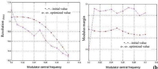
**Fig. 8.** (a) Resolution results for initial and optimized topology, (b) Modulus margin results for initial and optimized topology; (DAC delay:  $1.9T_s$ )
