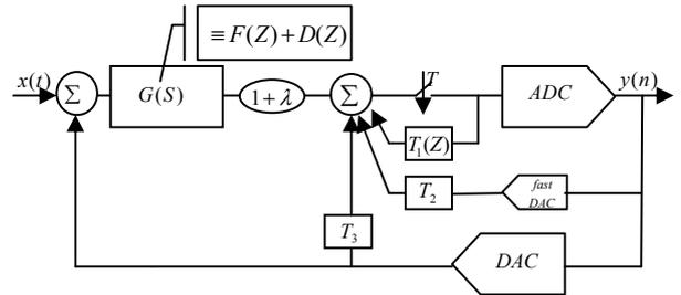
Fig. 1. Implementing a CT modulator with DAC delay
