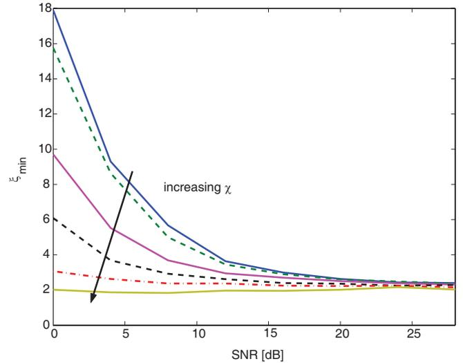
Fig. 2. Normalized antenna density  $\xi_{\min}$  above which dual-polarization should be favored as a function of the SNR ( $\chi^{-1}$  is the channel XPR,  $\chi \in \{0, 0.1, 0.3, 0.5, 0.7, 0.9\}$  and  $\delta_1 = \delta_2 = 0$ ).
