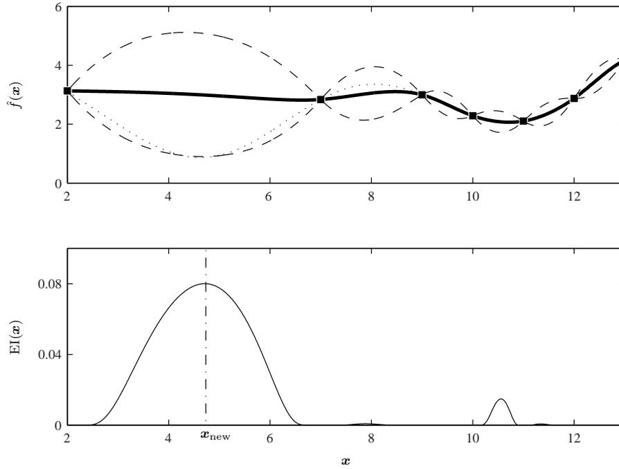
**Fig. 2** EI approach to optimization using Kriging: (*top*) prediction  $\hat{f}$  (bold line), 95% confidence intervals computed using  $\hat{\sigma}$  (dashed line) and true function  $f$  (dotted line); (*bottom*) expected improvement.
