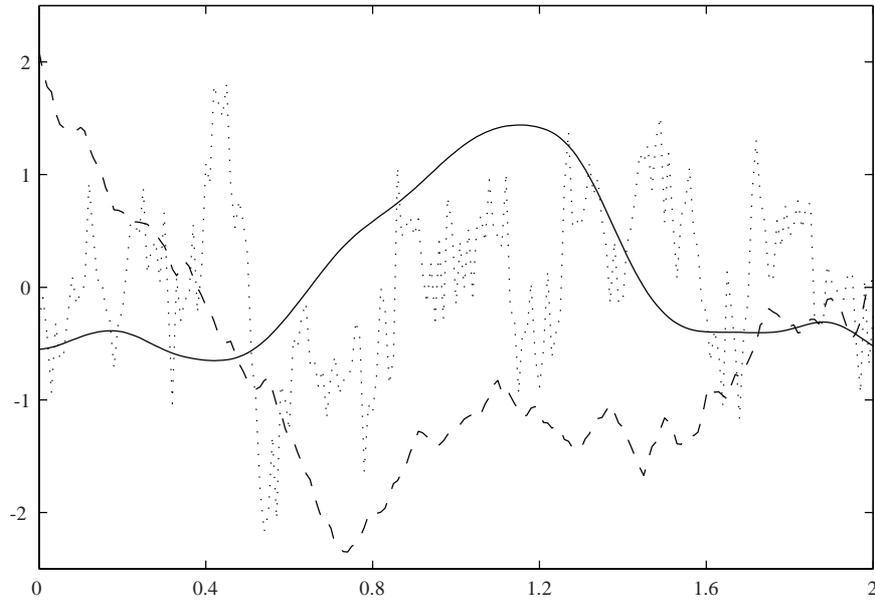
**Fig. 11** Three sample paths of a zero-mean Gaussian process with a Matérn covariance. Conventions are as in Figure 10:  $\nu = 4$  for the solid line,  $\nu = 1$  for the dashed line and  $\nu = 0.25$  for the dotted line.
