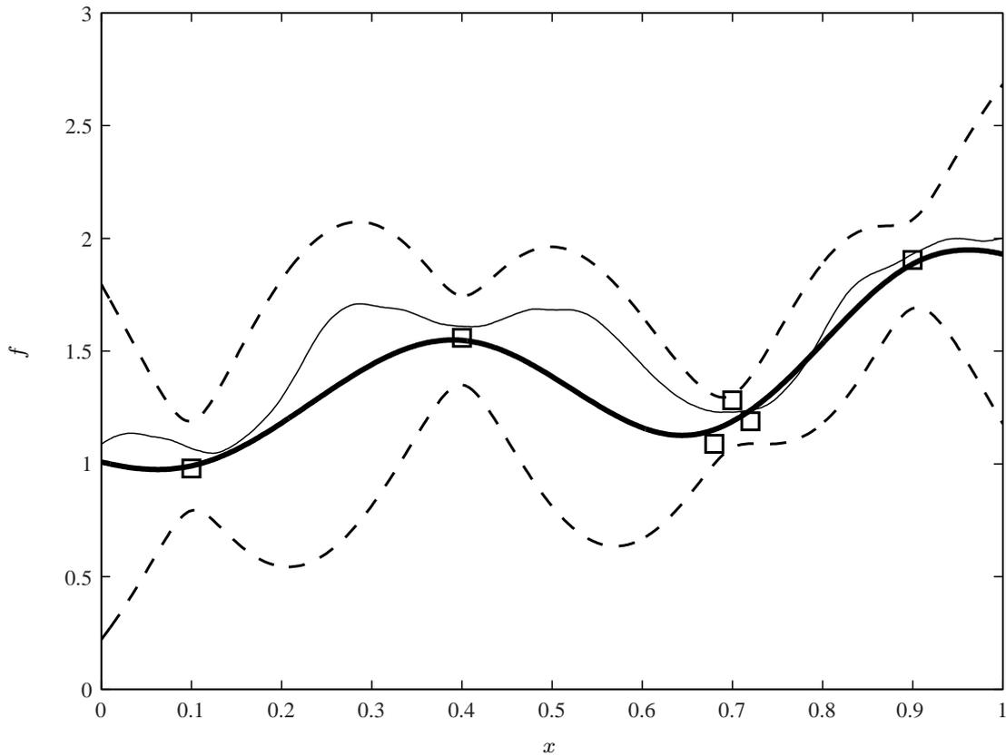
**Fig. 5** Example of prediction by Kriging (bold line) of noisy measurements represented by squares. Dashed lines represent 95% confidence regions for the prediction and the thin solid line is an example of conditional simulation obtained using the method presented in Section 5.3.1.
