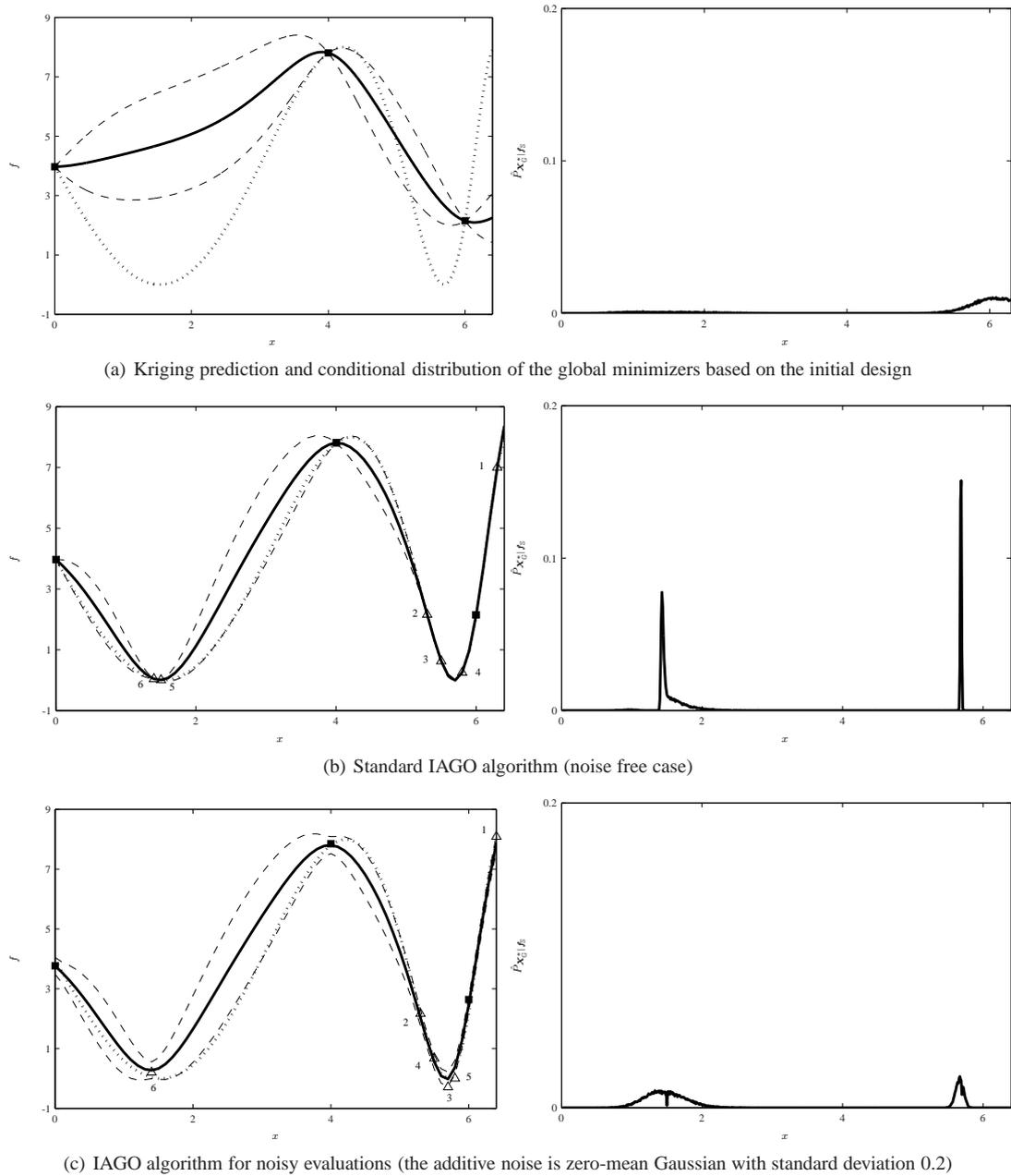
**Fig. 6** Example of global optimization using IAGO on a function of one variable (dotted line), with an initial design consisting of three points (represented by squares). Six additional evaluations are carried out (triangles) using two versions of the IAGO algorithm. The graphs on the *left part* of the figure account for the predictions, while the *right part* presents the corresponding conditional distributions of the global minimizers.
