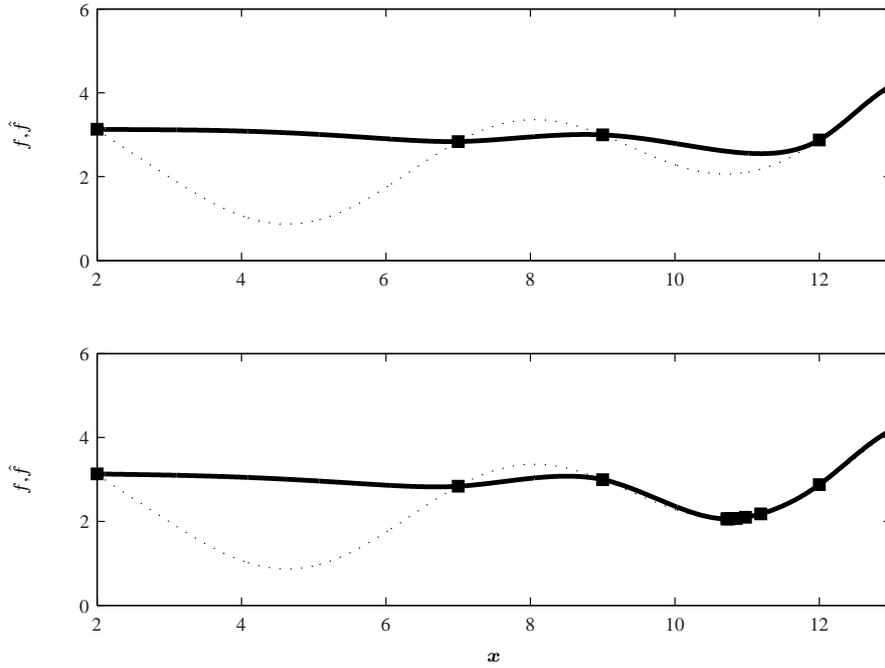
**Fig. 1** Naive approach to optimization using Kriging: (*top*) prediction  $\hat{f}$  (bold line) of the true function  $f$  (dotted line, supposedly unknown) obtained from an initial design materialized by squares; (*bottom*) prediction after seven iterations minimizing  $\hat{f}$ .
