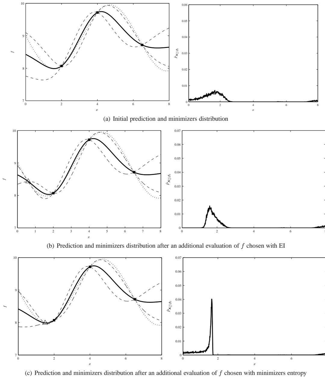
**Fig. 8** Comparison between minimizers entropy and EI: the *left* side contains the Kriging predictions before and after an additional evaluation chosen with either EI or minimizers entropy, while the *right* side presents the corresponding conditional distribution of the global minimizers.
