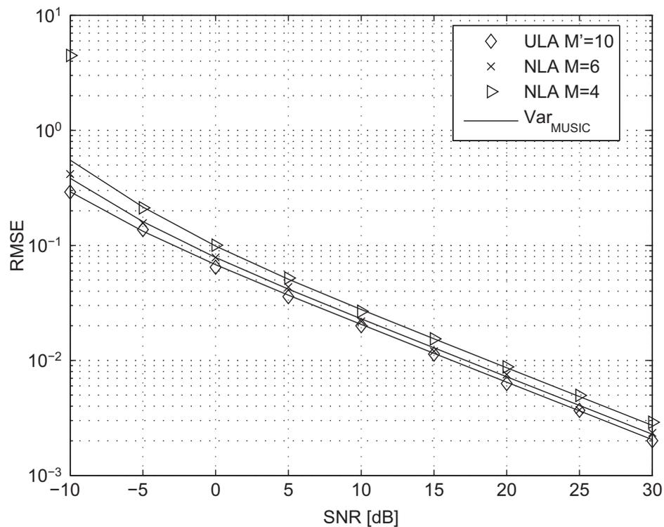
**Fig. 5.** RMS error for the source at  $-5^\circ$  with  $M' = 10$  in the case of ULA,  $M = 6$  and 4 in the case of NLA, DOA =  $[-5^\circ, 10^\circ]$ .
