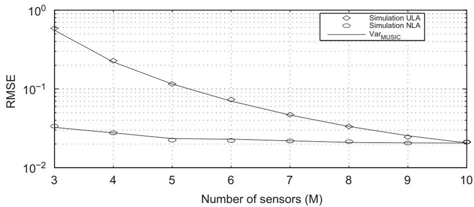
**Fig. 4.** RMS error for the source at  $-5^\circ$  with  $M = 3, 4, \dots, 10$ , SNR = 10 dB, DOA =  $[-5^\circ, 10^\circ]$  in the case of ULA and NLA.
