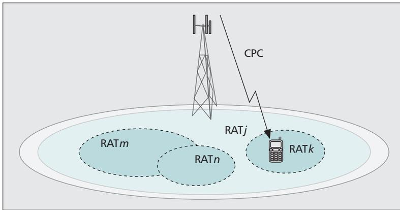
Figure 3. The CPC in a heterogeneous RAT environment.
