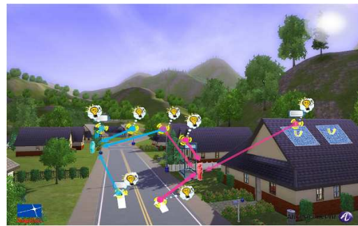
Fig. 1. Dense rechargeable base stations which coordinate their transmissions towards users by forming reconfigurable virtual antenna arrays.
