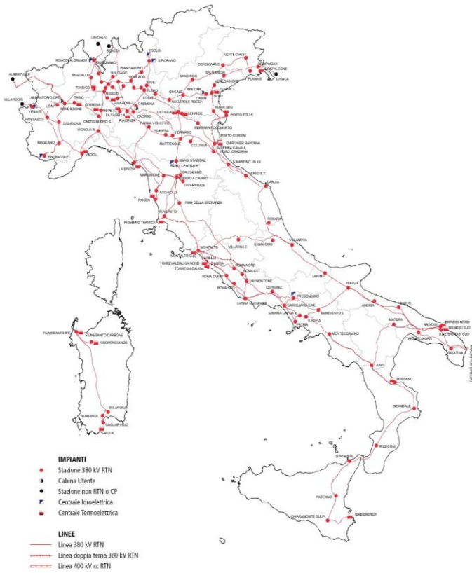
Figure 1. The 380 kV Italian power transmission network (TERNA 2002, Rosato et al. 2007)
