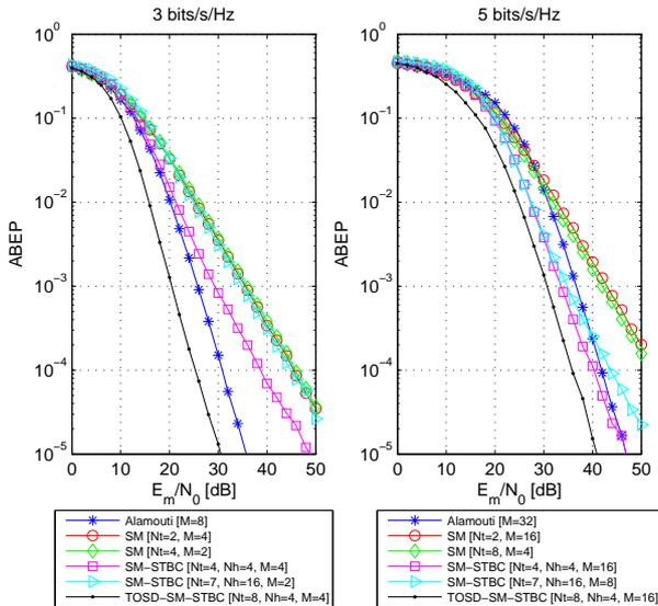
Fig. 1. ABEP against  $E_m/N_0$ . Performance comparison with SM [3] and Alamouti [18] schemes for a rate of 3 bits/s/Hz (left) and 5 bits/s/Hz (right).
