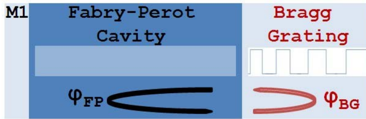
Figure 1. Schematic of a Continuum resonant cavity, in which the total round trip phase has been divided between the Bragg grating ( \varphi_{BG} ) and the rest of the cavity ( \varphi_{FP} )
