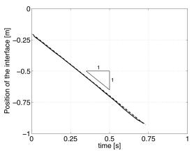
**Fig. 6** Influence of the mesh on the resolution of the Hamilton-Jacobi equation: position of the interface (black dot on figure 3) as a function of time for a constant velocity  $v_n = 1$  m/s, and for three different meshes: coarse mesh (solid line, figure 4(a)), fine mesh (dashed line, figure 4(b)), and most refined mesh (dotted line, figure 4(c))
