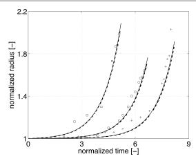
**Fig. 7** Value of the normalized radius of a pipe as a function of time computed using the level-set formulation described in this paper (thick dashed lines), using the analytical formula of [43], or using the experimental data from [20] (for tests MDHET006, WBHET001 and HD-HET007, respectively in squares, circles and pluses).
