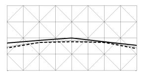
**Fig. 5** Influence of the mesh on the shape of the interface at t=20 s, starting from a sine profile: coarse mesh (solid line, figure 4(a)), fine mesh (dashed line, figure 4(b)), and most refined mesh (dotted line, figure 4(c)). Only the latter mesh is represented (gray lines). This figure is a zoom in the black boxes of figure 4
