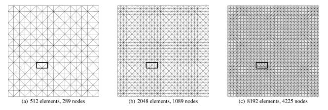
Fig. 4 Three different meshes; the black boxes indicate the zoom displayed in figure 5
