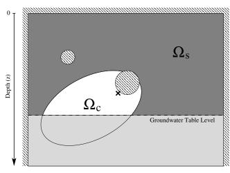
**Fig. 8** Modeling of a leaking duct: a cavity  $\Omega_c$  within a soil  $\Omega_s$ , with no outgoing flux on the left, right and upper sides, two ducts (the dashed holes), one of which leaking (at the location of the star), and a rising water table (dashed line and light grey shade)
