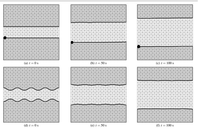
Fig. 3 Snapshots at different moments of the piping phenomenon, starting from a linear pipe (upper plots) or a pipe with a sine profile (lower plots). The black dots in the upper figures indicate the point that is being followed in the numerical test of figure 6
