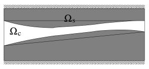
Fig. 2 Modeling of the piping phenomenon: a small channel  $\Omega_c$  in a mass of soil  $\Omega_s$  opens up under the eroding action of the water flowing from the right to the left.
