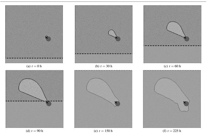
Fig. 10 Snapshots at different moments of the hollow (light grey shade) in the ground (dark grey shade) created by a leaking duct (the duct is the dark grey circle and the leak is the black cross). Before (d), the water table (dashed line) is below the hole in the duct and the jet model is used. After (d), the flow model is used.
