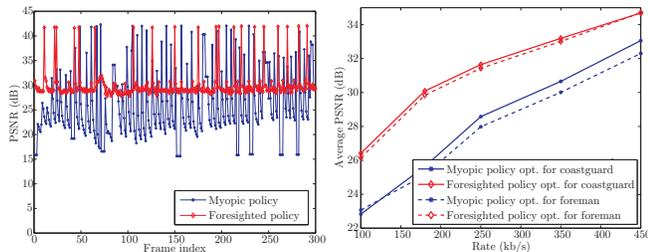
**Fig. 3.** Evolution of the PSNR as a function of time (left) and channel rate (right) for the coastguard.qcif sequence when  $\pi_m^*(s)$  and  $\pi_f^*(s)$  optimized for the foreman.qcif sequence (dashed) and when  $\pi_m^*(s)$  and  $\pi_f^*(s)$  optimized for the coastguard.qcif sequence (plain)
