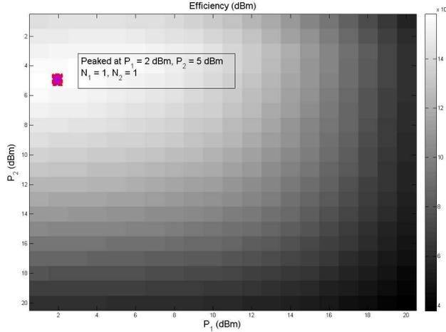
Fig. 2.  $\eta$  over combinations of  $P_1$  and  $P_2$  with  $\frac{b}{\sigma_1^2} = 100$  (20dB),  $N_1 = N_2 = 1$ . Zone 2 corresponds to a lower SINR and in this case the efficiency is optimized by using more power on the zone 2 user.
