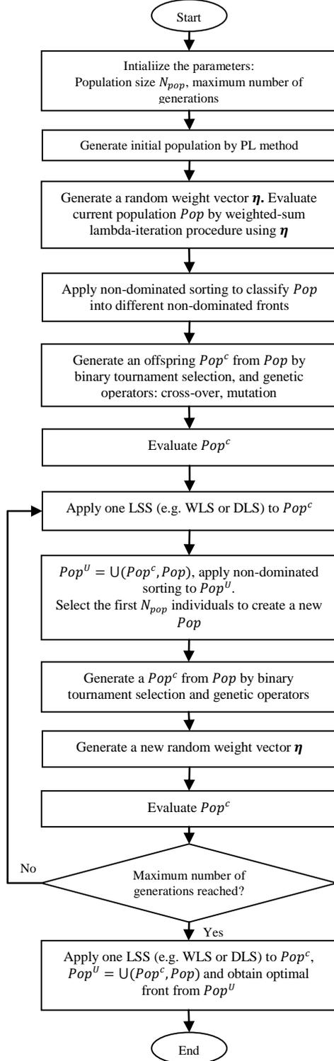
Figure 3. Flow chart of NSGA-II + LSA
