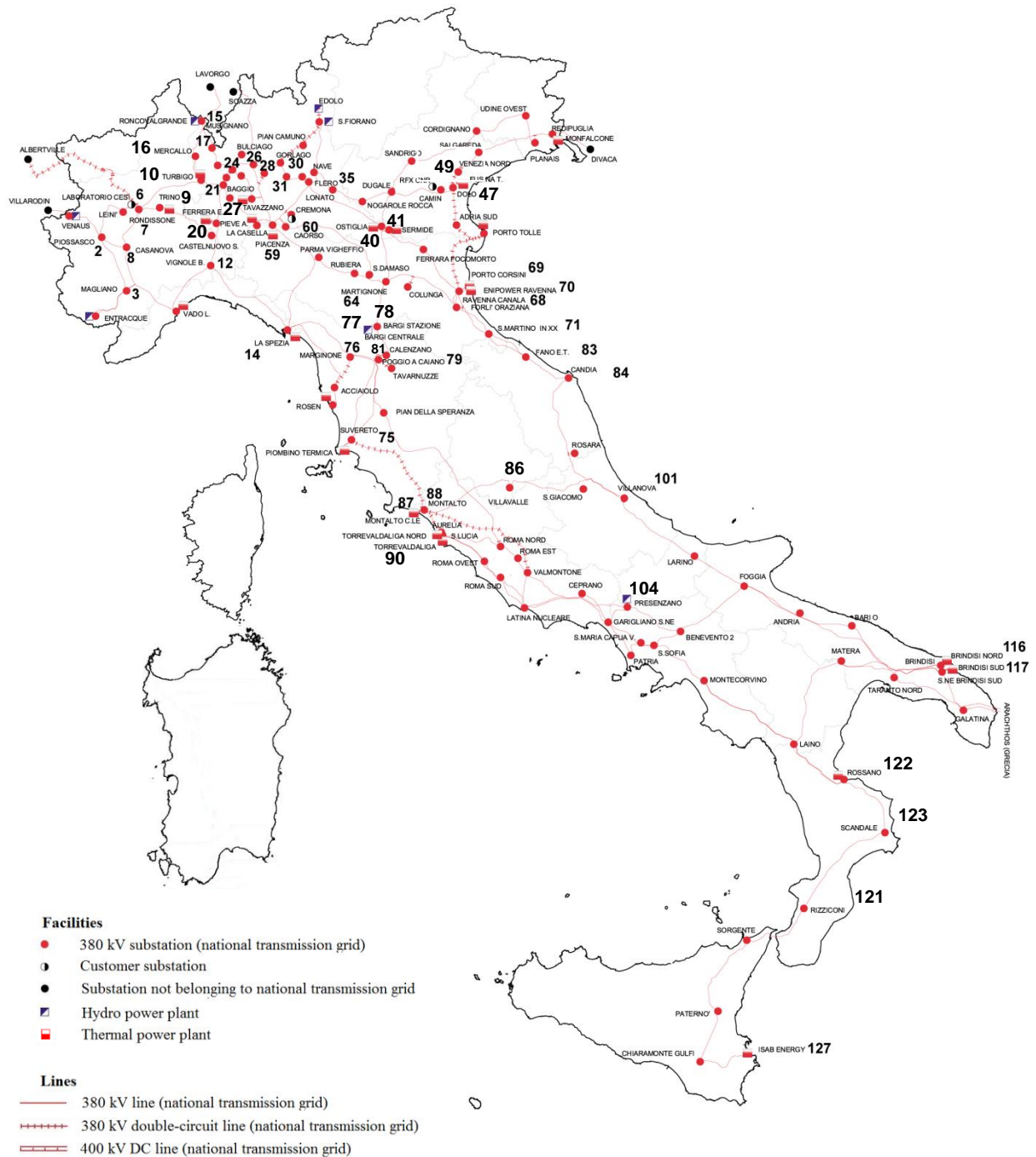
Figure 1. The 380 kV Italian power transmission network [TERNA, 2002; Rosato et al., 2007]
