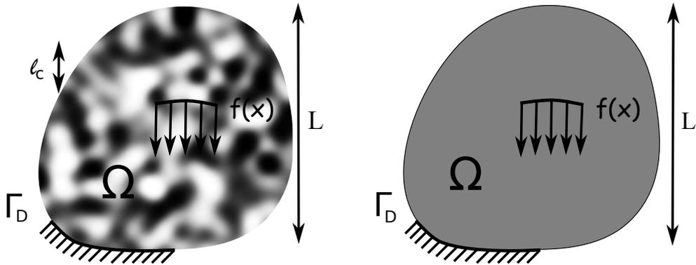
Fig. 2. Description of one realization of the random medium (left), with fluctuating coefficient  $\mathbf{k}_\varepsilon(x)$ , and corresponding effective medium (right), with constant deterministic effective tensor  $K^*$ .
