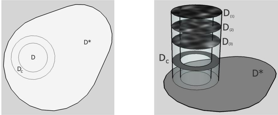
Fig. 1. Section (left) and perspective view (right) of a 2D Arlequin problem where an effective model, defined over domain  $\underline{D}$ , and several realizations of a random model, defined over  $D$ , are coupled through a coupling domain  $D_c$ . On the overlap outside of  $D_c$ :  $(D \cap \underline{D}) \setminus D_c$ , both models are defined but behave independently.
