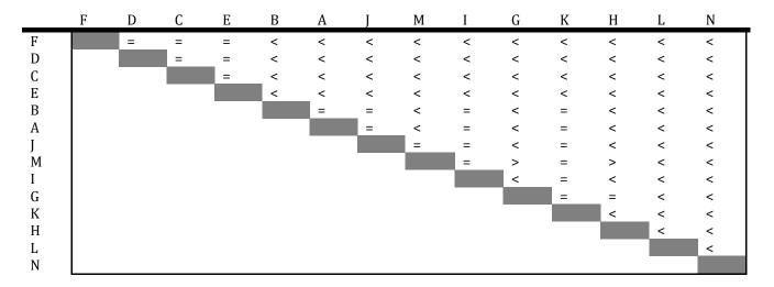
Table reports the results obtained in [19] applying the probabilistic approach to the same case study. The main difference is that the probabilistic approach results in fewer cases of components with the same importance because the CDFs of the components' important measures appear to be more clearly separated than are the necessity and possibility measures in the possibilistic approach.
