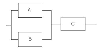
Fig. 1. System Reliability Block Diagram.
