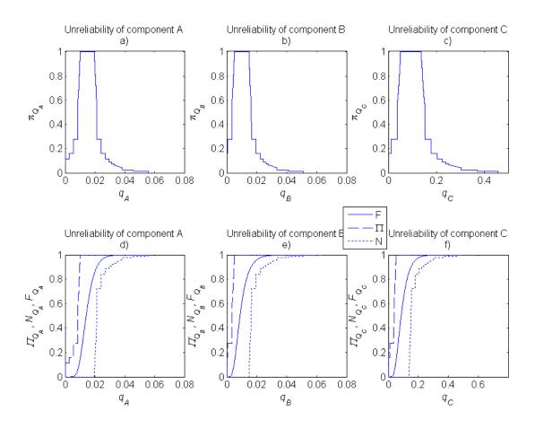
Fig. 4. a,b,c: possibility distributions of the unreliabilities of the components A,B, and C, respectively. d,e,f: possibility (dashed lines), and necessity (dotted lines) measures of the corresponding component unreliabilities. The continuous lines refers to the CDF of the component unreliability obtained in Section 2 in the probabilistic framework. The scales of the abscissas of a and b are different from that used in c.
