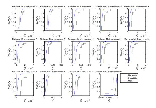
Fig. 8. Possibility, and necessity measures of the components' Birnbaum IMs (reported in different scales.). The continuous line refers to the CDFs obtained in the probabilistic case [14].
