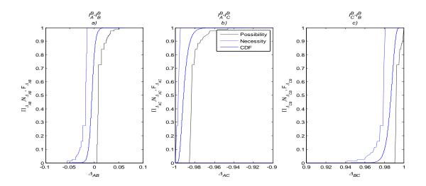
Fig. 3. Comparison of the possibility measure, necessity measure, and CDF of the variables  $\Delta_{ki}$  k, j=A, B, C and  $k \neq j$ .
