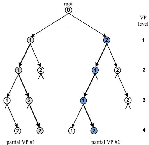
Fig. 4 An example of the proposed parallel QRDM encoder for  $p = 2$ ,  $G = M_G = T = 2$ , and  $K = 4$ .
