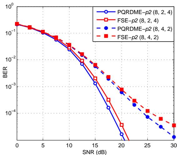
**Fig. 8** BER performance of the proposed PQRDME- $p2$  for  $M_G = T = 3$ , and a  $(n_T, n_U, n_R)$  MU-MIMO system.
