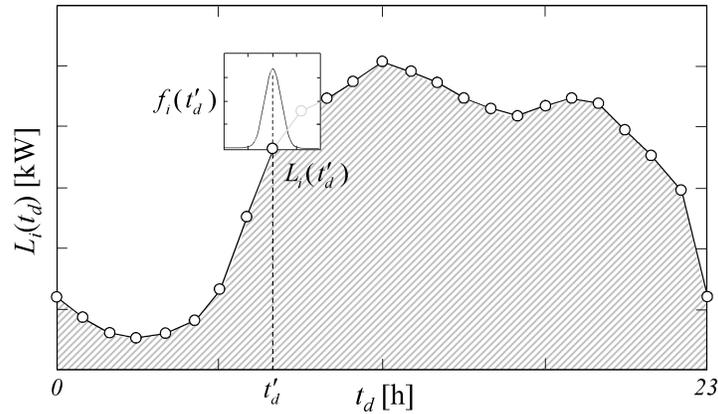
Figure 3. Daily load profile. Hourly normally distributed load
