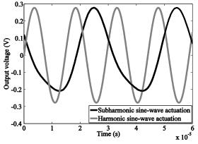
*Fig.* 2:Experimentalshape of the output close to resonance with subharmonic actuation (dark line) and harmonic actuation (grey line). On the dark line, the largefeedthrough signal (frequency  $f_0$ /2)overshadows the small amplitude motional signal (frequency  $f_0$ ). A spectrum analyzer or a large-resolution ADC would be needed to extract the motional signal.
