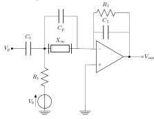
**Fig. 3:** Test circuit. The  $X_m$ -element is the resonator.  $V_b=10V$  is the bias voltage and  $V_p$  the 2V-amplitude and 150ns-width pulses.  $C_t=1\mu F$ ,  $R_t=1k\Omega$ ,  $C_1=10pF$  and  $R_1=1.0M\Omega$ .  $C_p$  is the unknown parasitic capacitance.
