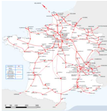
Figure 1. The 400kV French power transmission network
