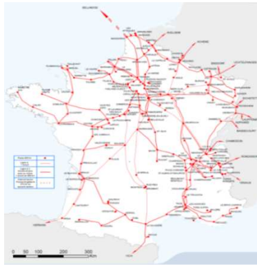
Figure 1. The 400kV French power transmission network
