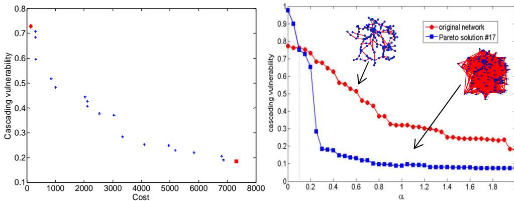
**Figure 2. (a) Pareto front reached by a population of 25 chromosomes evolving for 300 generations; (b) Comparison of the cascading vulnerability between the original and the most resilient networks under different network tolerance values**
