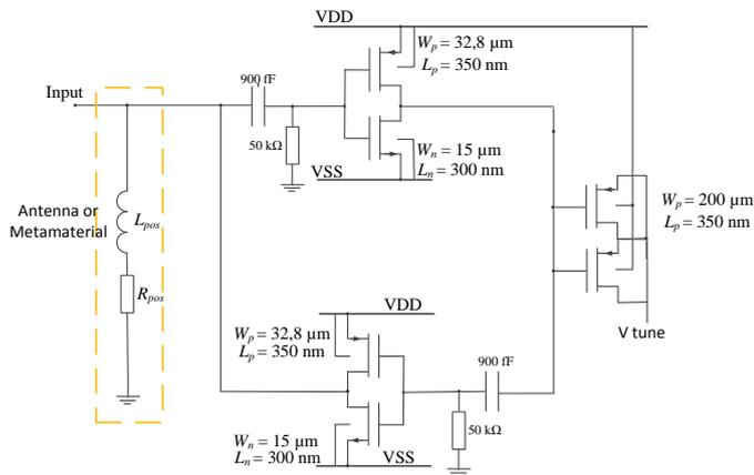
Fig. 4. Transistor level schematic of the circuit
