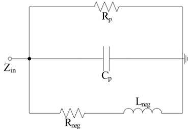
Fig. 2. The equivalent circuit of the gyrator
