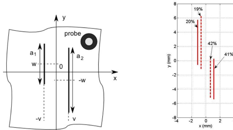
Fig. 1 *Left*: top view of the plate with the two parameterized cracks and the scanning probe. *Right*: reconstruction results in a test case. Solid/dashed lines: real/found cracks. Depths are shown in percentage of the plate thickness.
