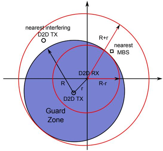
Fig. 3. Guard zone with radius  $R$  of a typical active D2D transmitter centered at the origin with its intended receiver being at distance  $r$  when  $R \geq r$ . According to the system model, no MBS or other active D2D transmitter can lie in a circle of radius  $R$  centered at the origin, thus the minimum distance from the nearest MBS or D2D transmitter to the typical active D2D receiver is between  $R - r$  and  $R + r$ .
