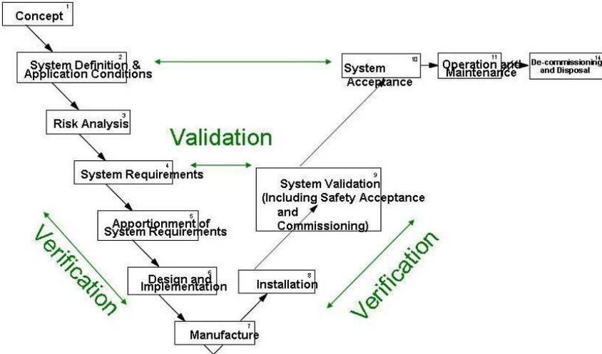
**Figure 1 - Railway systems V-Cycle according to EN 50126**
