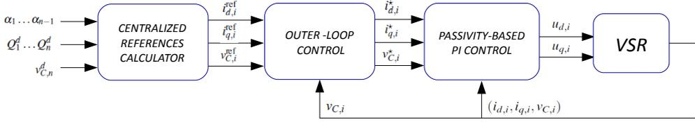
Figure 7: Control architecture of HVDC transmission systems under nominal operating conditions.
