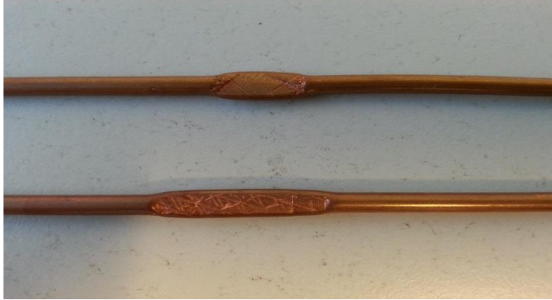
Figure 3 The two soft faults considered in the test whose severity depends on the length of crushing of the 30-cm semi-rigid cables.
