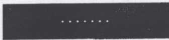
Figure 7: Spatial distribution of the line-of-points source produced by the optical holographic grating
