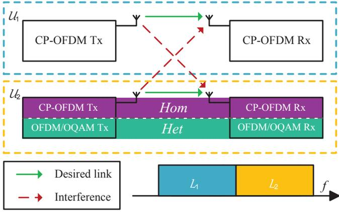
Fig. 1: Summary of the study led in the paper : two users  $\mathcal{U}_1$  and  $\mathcal{U}_2$  transmit on adjacent bands  $\mathcal{L}_1$  and  $\mathcal{L}_2$  and interfere with each other. Channel is assumed perfect and no Gaussian noise is considered.  $\mathcal{U}_2$  uses CP-OFDM in *Hom* scenario and OFDM/OQAM in *Het* scenario.
