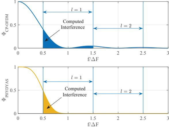
Fig. 3: Modeling of injected interference with the PSD-based model for CP-OFDM (top) and OFDM/OQAM with PHYDYAS filter (bottom). The values of interference injected by subcarrier 0 on a subcarrier at a spectral distance of  $l = 1$  correspond to the integration of the PSD from  $0.5 \Delta F$  to  $1.5 \Delta F$ .
