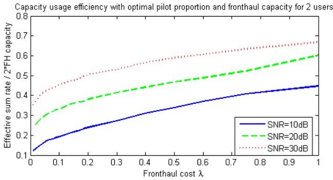
Fig. 4: Efficiency of capacity usage w.r.t. fronthaul cost
