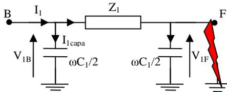
Figure 1. PI model of line section from protection to fault – Positive sequence network
