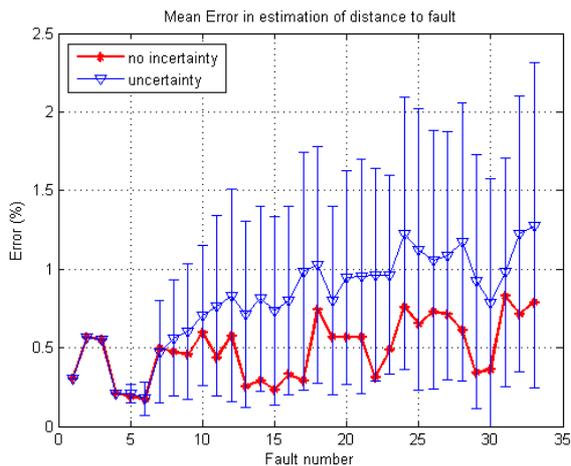
Figure 7. Relative error in fault distance estimation – Impact of load uncertainty
