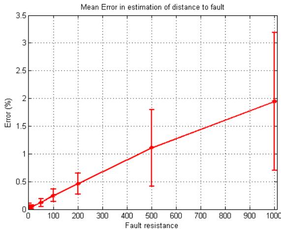
Figure 6. Relative error in fault distance estimation
