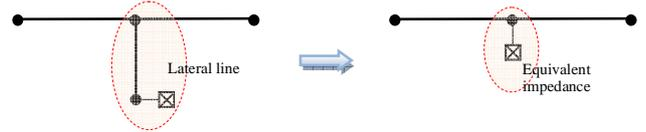
Figure 4. Estimation of measurements in case of lateral lines
