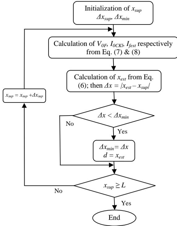
Figure 3. Fault location algorithm on homogeneous feeder
