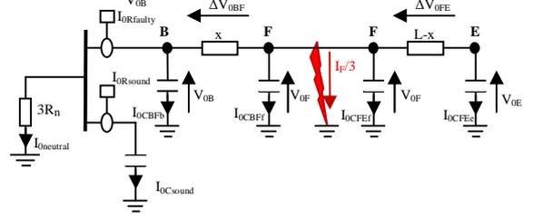
Figure 2. Generic zero-sequence network of MV distribution grids
