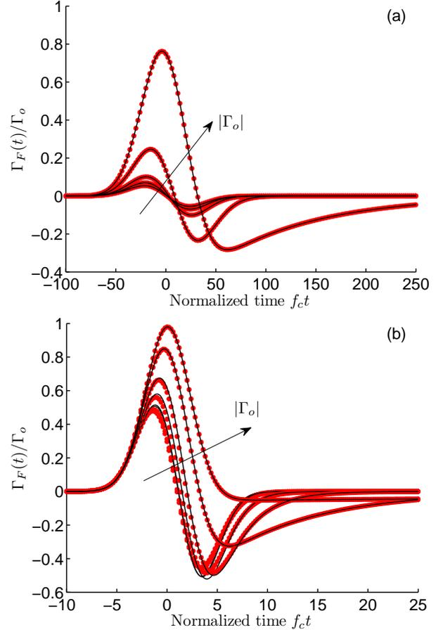
Fig. 4. Normalized time-domain echoes for an electrically-short fault, expected for a baseband Gaussian test signal with (a)  $B_o/f_c = 0.01$  and (b)  $B_o/f_c = 0.1$ . The different curves correspond to increasing values of  $\Gamma_o$  equal to 0.1, 0.2, 0.5, 0.7, 0.9 and 0.99, according to the direction of the arrows. Exact results (black solid lines) and approximations from the zero-pole model (red dots) are shown.
