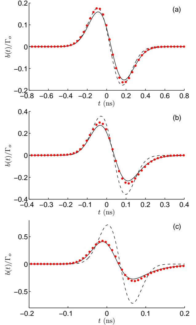
Fig. 9. Validation of the zero-pole model (9) and the derivative model (16), for the fault in Fig. 7(b) submitted to a Gaussian test signal with : (a)  $B_o = 1.25$  GHz, (b)  $B_o = 2.5$  GHz and (c)  $B_o = 5$  GHz. Numerical results are shown as red circles, predictions from the zero-pole model as solid black lines and for the derivative model as dashed lines. The critical frequency is  $f_o = 3.16$  GHz.
