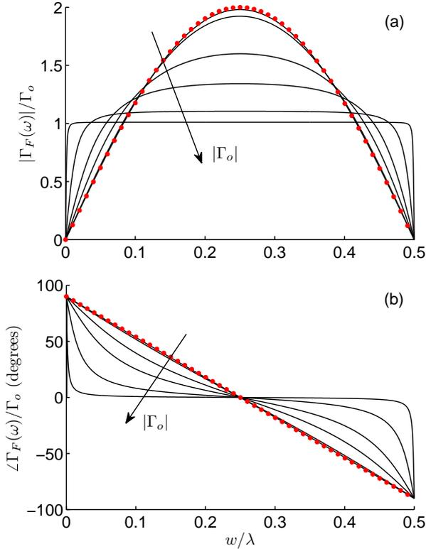
Fig. 2. Amplitude and phase-shift angle for the echo response  $\Gamma_F(\omega)$  predicted by (7), for six values of  $|\Gamma_o|$ , namely 0.1, 0.2, 0.5, 0.7, 0.9 and 0.99, in increasing order according to the direction of the arrows in the graphics. The red dots represent the soft-fault (weak perturbation) approximation (8).
