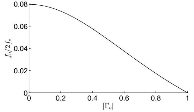
Fig. 6. Maximum normalized frequency  $f/f_c$  for which the derivative approximation holds, as a function of the fault severity  $|\Gamma_o|$ , evaluated taking a safety factor 2 below the frequency  $f_o/f_c$  in the condition (15).
