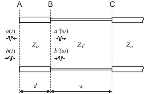
Fig. 1. Double impedance-step representation of a local fault in a transmission line of characteristic impedance  $Z_o$ , and relevant quantities for the derivation of the response  $\Gamma_F(\omega)$  of a fault of impedance  $Z_F$ .
