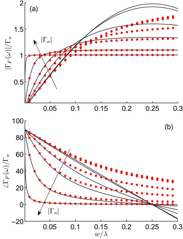
Fig. 3. Comparison of the exact (black solid lines) and zero-pole (red dots) models for the fault echo response  $\Gamma_F(\omega)$ . Six different values of  $\Gamma_o$  are shown, 0.1, 0.2, 0.5, 0.7, 0.9 and 0.99, in increasing order according to the direction of the arrows in the graphics.
