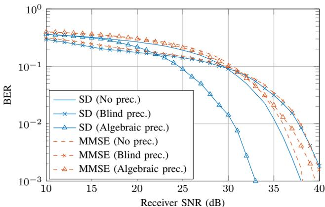
Fig. 3. Comparison of the average stream bit error rate (BER) for an *unknown* DP LoS MIMO ULA channel at the transmitter, with inter-antenna distance  $d = 0.33d_{\text{opt}}$  and different decoding and precoding architectures. Each stream supports a 64-QAM, with thus 6 bits per stream.
