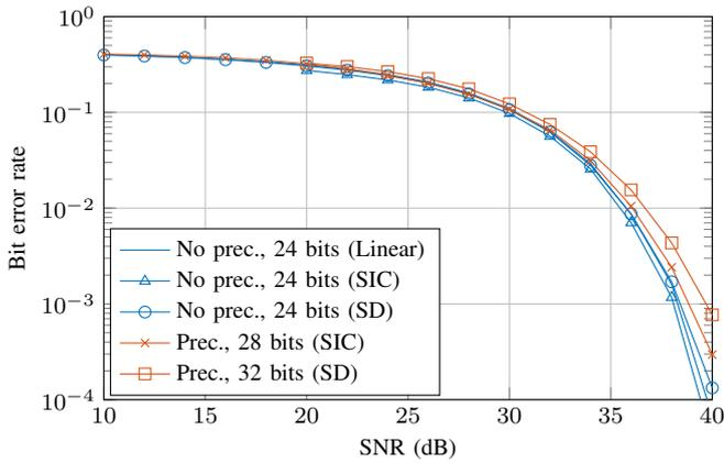
Fig. 2. Comparison of the average stream bit error rate (BER) for an *known* DP LoS MIMO ULA channel at the transmitter, with inter-antenna distance  $d = 0.33d_{\text{opt}}$  and different decoding and precoding architectures. The rate of each stream is adapted when precoding is used, as to achieve a BER of  $10^{-3}$ .
