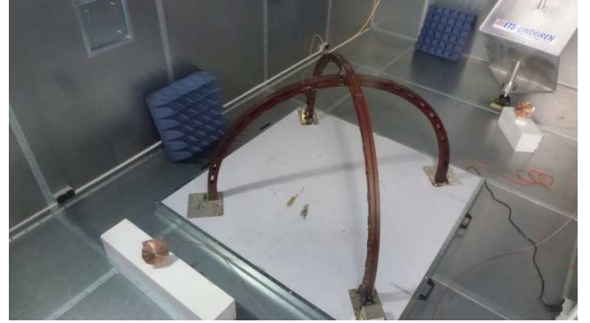
Fig. 6: The robot as tested in the reverberation chamber, with two of the absorbers used in order to control the spread time of the chamber.
