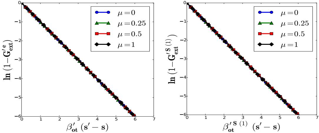
Figure 3: Extinction cumulative distribution functions associated with the transparent propagation phase between overlapping opaque cylinders (OT Beerian case); Left:  $G'_{ext}$  issued from random isotropic volume points, equal to  $G^S_{ext}(\mathbf{u}, s' - s)$  associated with a diffuse reflection law; Right:  $G'^S_{ext}^{(1)}$  associated with the first set of scattered rays following a Fresnel's law.
