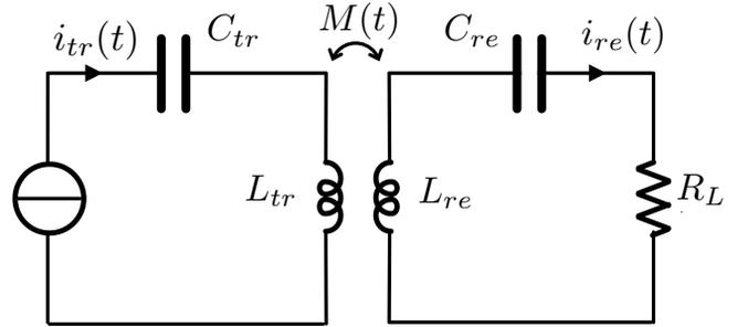
Fig. 5: Circuit representation of the analyzed configurations.
