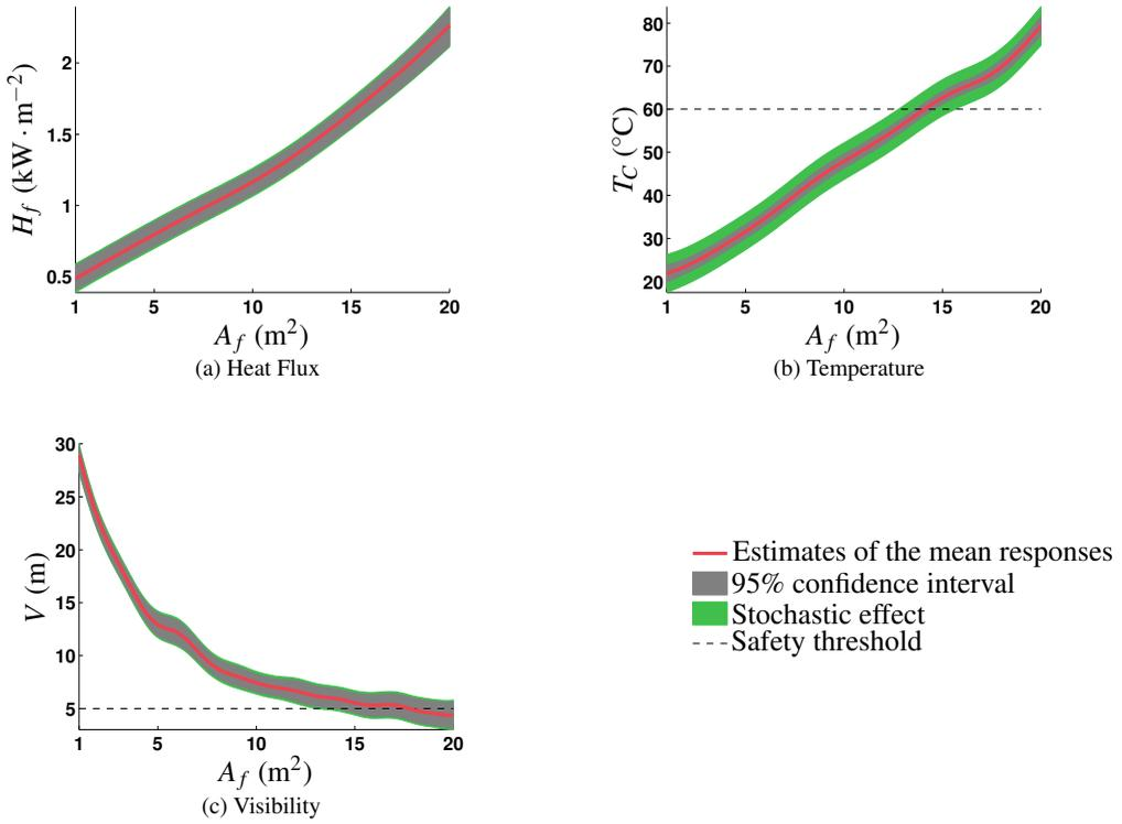
Fig. 5. Estimates of the three outputs as function of the fire area  $A_f \in [1; 20]$  m<sup>2</sup>. (a) Heat Flux  $H_f$ . (b) Temperature  $T_c$ . (c) Visibility  $V$ . The safety threshold of  $H_f$  is never reached.
