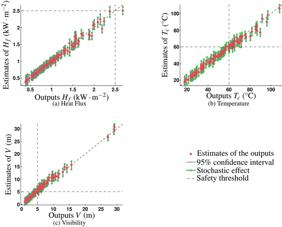
Fig. 7. Comparison between estimates (ordinate) and high-fidelity simulations (abscissa), for the three outputs: (a) Heat Flux  $H_f$ , (b) Temperature  $T_c$  and (c) Visibility  $V$ . The dashed diagonals are the lines  $y = x$ .
