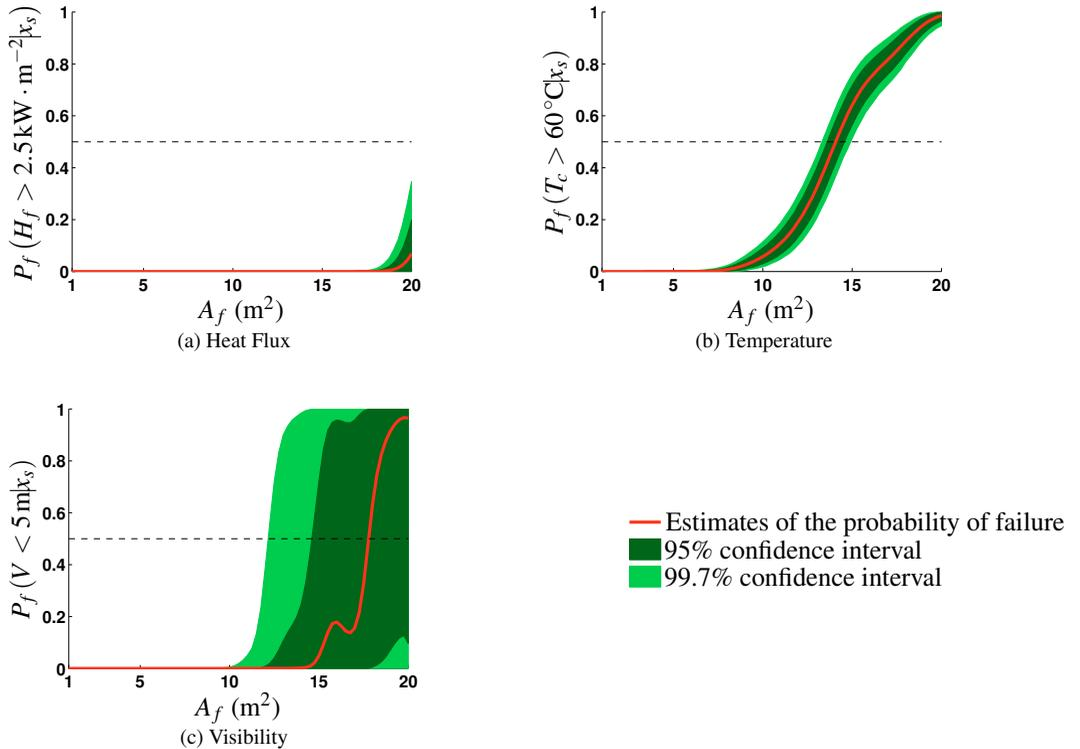
Fig. 6. Estimates of probabilities of failure as function of the scenario variable  $A_f \in [1; 20]$  m<sup>2</sup>, the fire area. Each figure corresponds to one output: (a) Heat Flux  $H_f$ , (b) Temperature  $T_c$  and (c) Visibility  $V$ .
