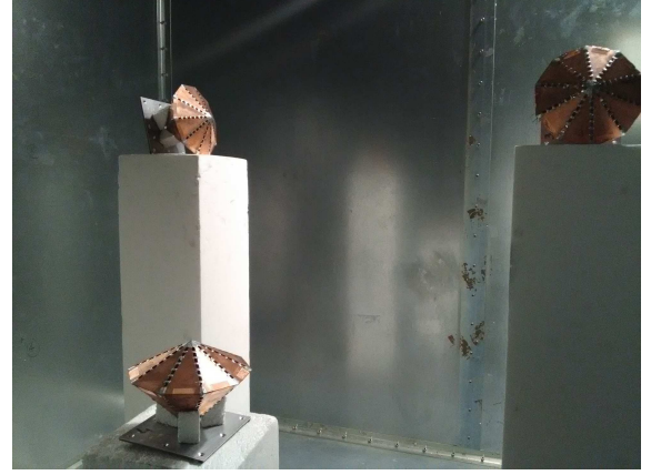
Fig. 2: Part of the experimental setup, with three of the loading antennas mounted on top of styrofoam supports.
