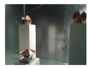
Fig. 2: Part of the experimental setup, with three of the loading antennas mounted on top of styrofoam supports.
