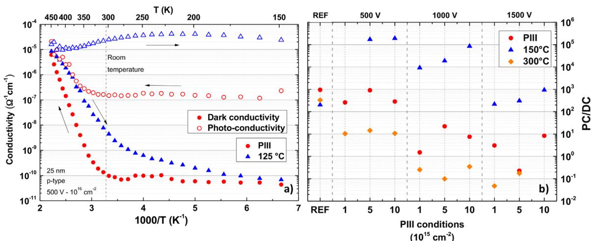
**Figure 4.** (a) Dark- (DC) and photo- (PC)-conductivity measurement after a 500 V and  $10^{16} \text{cm}^{-2}$  PIII  $\text{B}_2\text{H}_6$  implantation against temperature. (b) Room temperature photosensitivity after each process step and against different PIII implantation conditions. For this latter experiment only, a 630 nm illumination at a flux of  $2.6 \times 10^{16} \text{cm}^{-2} \text{s}^{-1}$  is used.
