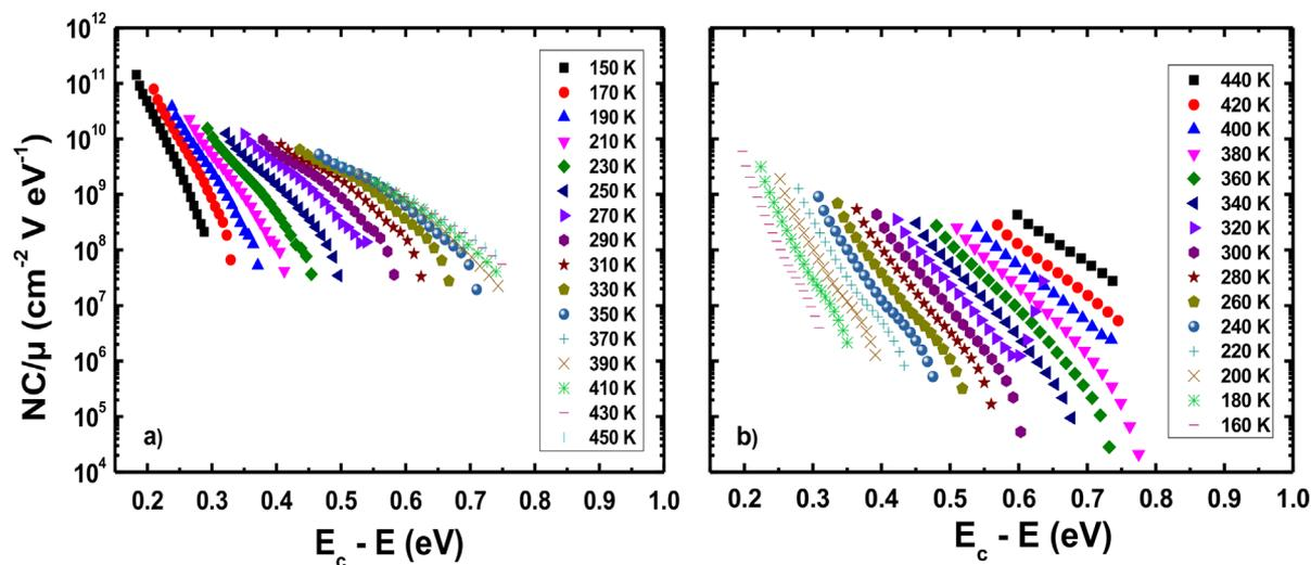
**Figure 3.** MPC measurement results of a-Si:H layer with a B<sub>2</sub>H<sub>6</sub>-PIII at 500V and 10<sup>16</sup> cm<sup>-2</sup> (a) after PIII and (b) after PIII and annealing at 440 K for 60 min.
