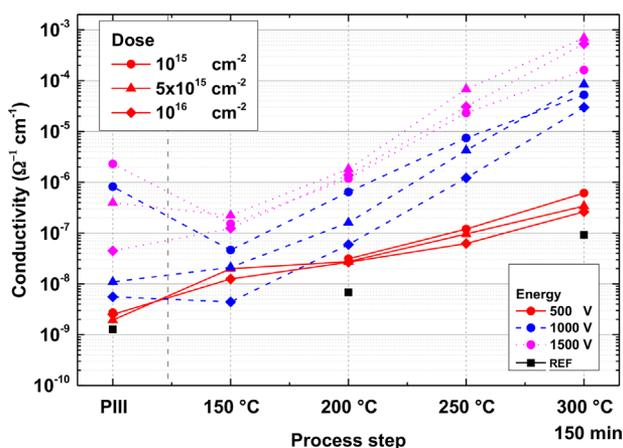
**Figure 2.** Measured effective room temperature conductivity of (p) a-Si:H layers implanted at different energies and doses (see Figure 1), after each process step: just after implantation (PIII) and after subsequent annealing steps at increasing temperatures (150, 200, 250, and prolonged annealing at 300 °C). For the reference sample, the conductivity before annealing is reported at the PIII step.
