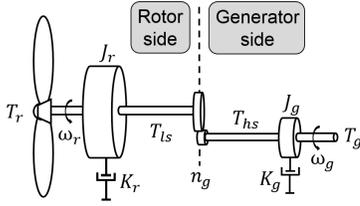
Fig. 1: Two-mass model of the turbine mechanics.
