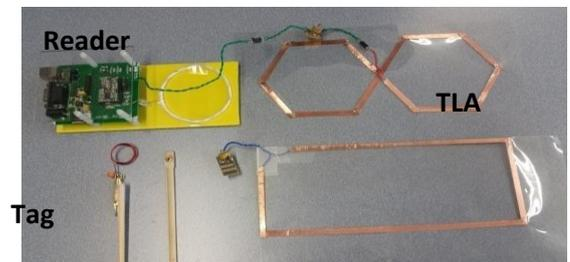
Fig 9. Experimental setup for RFID detection tests
