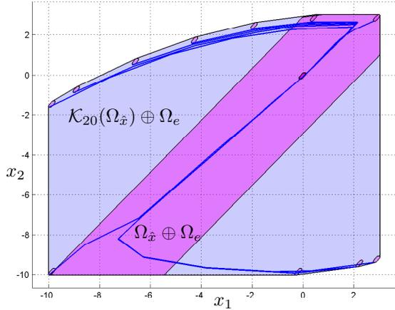
Fig. 1. Maximal output admissible set  $\mathcal{K}_{20}(\Omega_{\hat{x}}) \oplus \Omega_e$  and the closed-loop dynamics of system (1).
