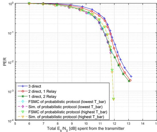
Fig. 6. Achievable PER with deterministic and probabilistic protocols
