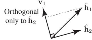
Fig. 1. If the pilot-contaminated channel estimates are linearly independent (i.e., not parallel), there exists a combining vector  $\mathbf{v}_1$  that rejects the pilot-contaminated interference from UE 2 while  $\mathbf{v}_1^H \hat{\mathbf{h}}_1 \neq 0$ .
