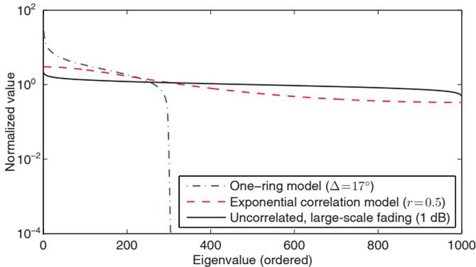
Fig. 3. Average eigenvalue distribution with three channel covariance models, whereof one gives a rank-deficient matrix and the others have full rank.
