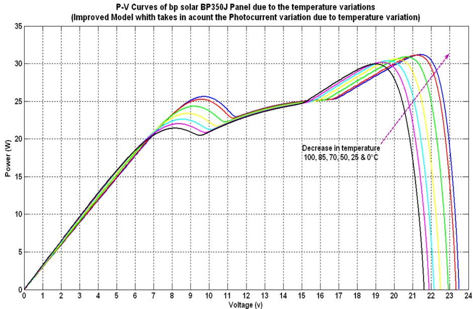
**FIGURE 8.** Displacement of the local MPP on the P-V characteristics of the BP350J solar panel under partial shadow and temperature changes.
