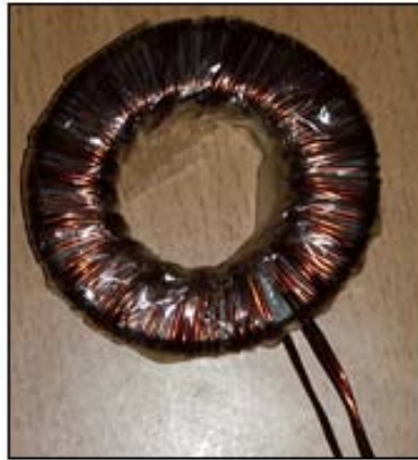
Figure 9. Realized coil of 2,48 mH.
